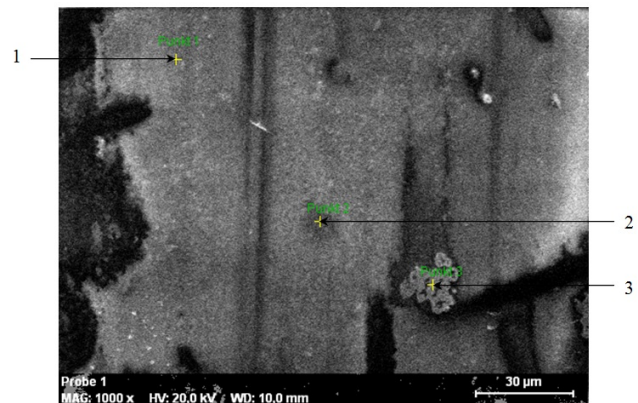
Fig. 4. Chemical analysis of tribosurface of epoxycomposite of composition No. 6
