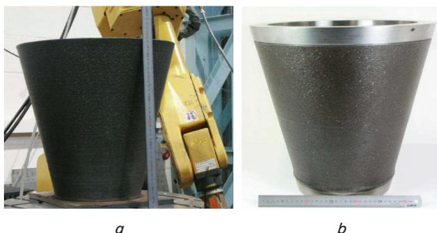
Fig. 4. Manufacturing of thin-walled conical parts of stainless steel [17]: *a* – before machining; *b* – during machining (the height of the parts is – 1 m, the biggest diameter is 0.5 m)
