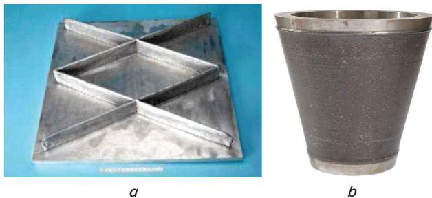
Fig. 3. Examples of three-dimensional products from carbon steel S355 [17]: *a* – panels with intersecting ribs without machining; *b* – part, machined after manufacturing
