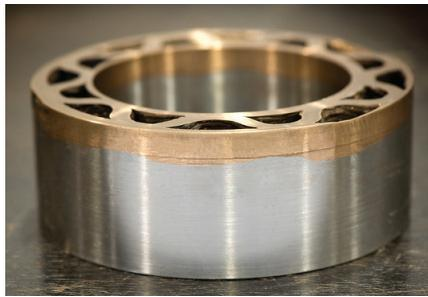
Fig. 7. Volumetric hollow part with internal stiffeners made of bimetal «structural steel – bronze Cu-3 % Si», obtained by means of arc welding (cladding) with current-carrying wire [17]
