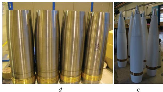
Fig. 6. Production of complex profile parts with variable wall thickness from high-strength steels using the example of the shell body (height – 800 mm, diameter – 160 mm, wall thickness 18–8 mm, weight – 32 kg, productivity 4 kg/h [17]: *a* – the initial stage; *b* – cylindrical section; *c* – conical section; *d*, *e* – finished parts
