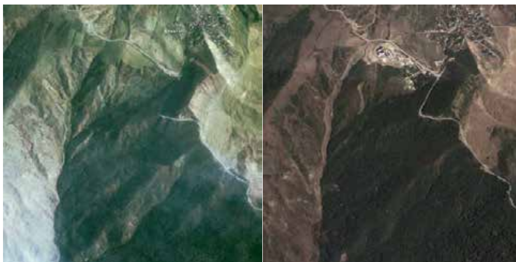
Fig.3. Retrospective analysis of landslide formation. a) satellite image of 2004, b) satellite image of 2012 The landslide began to form after the construction of the tourist complex
