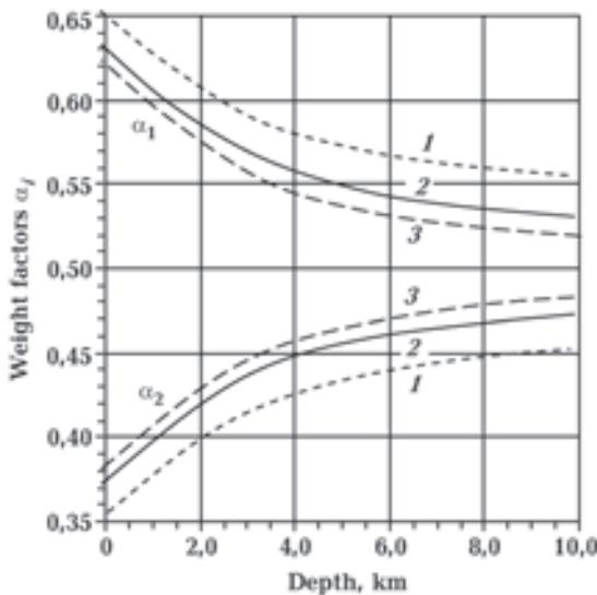
Fig. 6. Weight factors  $\alpha_i$  vs depth occurrence of reservoir: 1 — dolomite, 2 — limestone, 3 — sandstone.
