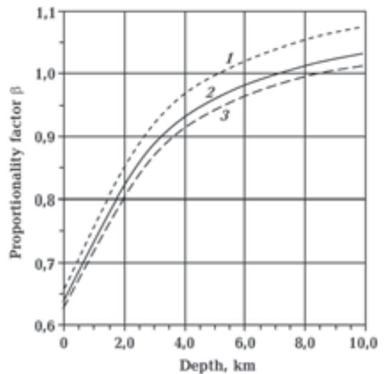
Fig. 9. Proportionality factor  $\beta$  vs depth occurrence of reservoir: 1 — dolomite, 2 — limestone, 3 — sandstone.
