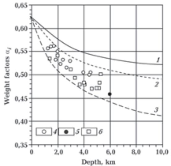
Fig. 7. Weight factor  $\alpha_1$  for sandstone. Pressure gradient: 1 — 10 MPa/km (CHP), 2 — 13 MPa/km (lower limit of AHFP), 3 — 23 MPa/km (upper limit of AHFP). Examples of AHFP: 4 — DDD [Melik-Pashaev et al., 1983], 5 — DDD [Lukin, 2014b]; 6 — other regions of the world [Petrenko et al., 2004].
