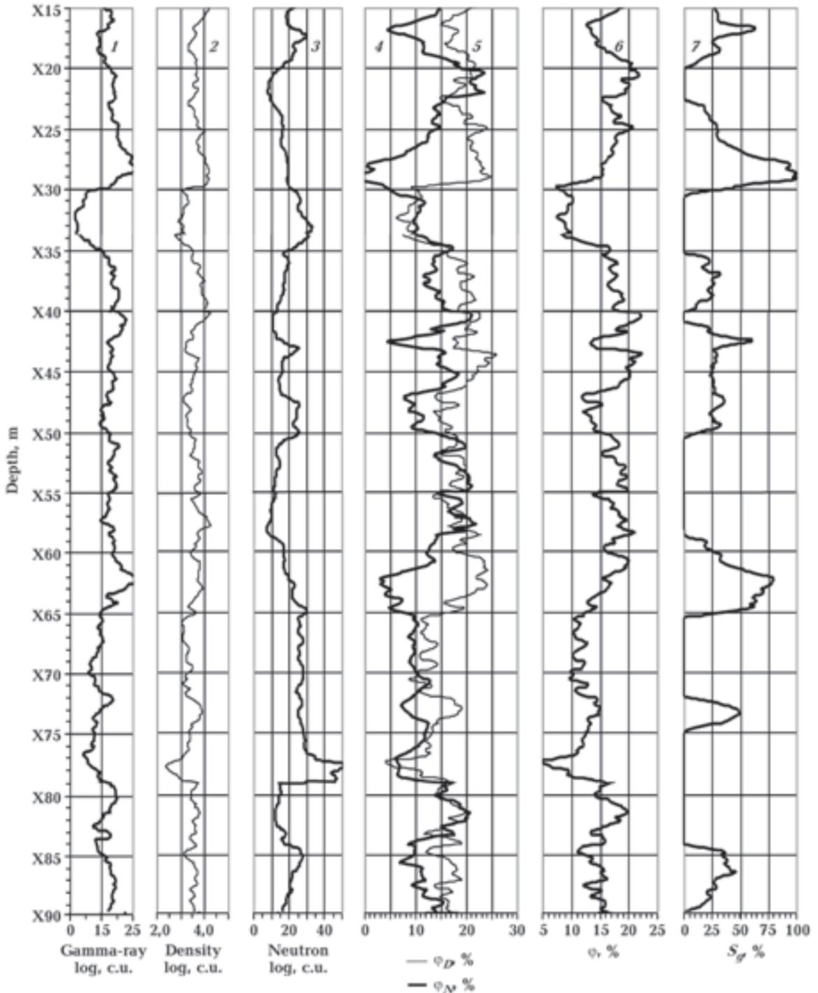
Fig. 4. Diagrams of radioactive logging (1 — gamma-ray log, 2 — density log, 3 — neutron log; c. u. — conventional unit) and petrophysical parameters of formations (4 — neutron porosity, 5 — density porosity, 6 — true porosity, 7 — gas saturation) obtained in coalbed methane well (Donbas, terrigenous geologic section).
