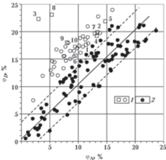
Fig. 5. Field example of neutron-density porosity crossplot: 1 — gas reservoir, 2 — water reservoir; 1—10 — number of gas reservoirs in Tab. 1.
