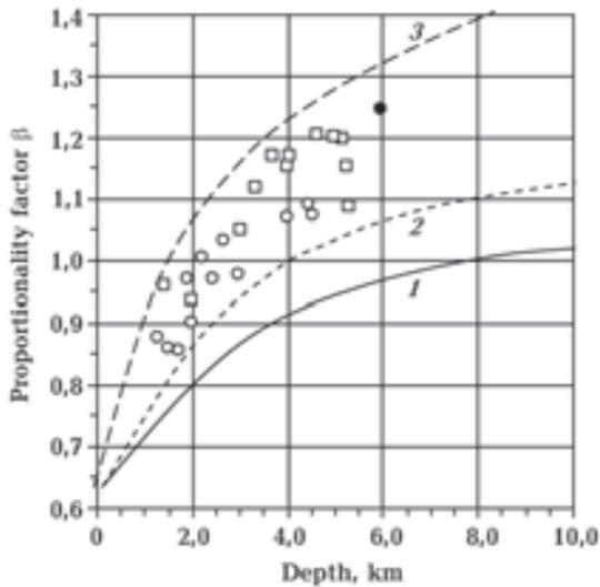
Fig. 10. Proportionality factor  $\beta$  for sandstone. Legend see in Fig. 7.
