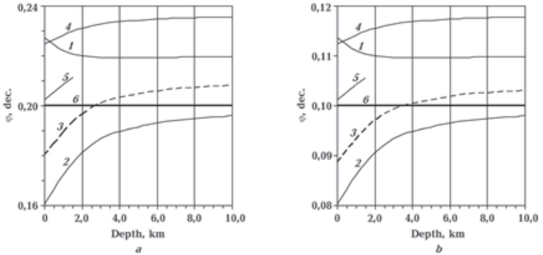
Fig. 8. Porosity of gas reservoir from density-neutron log porosity vs depth by: 1 — root-means-square equation (14); 2 —  $\alpha_1=0.50, \alpha_2=0.50$  (Eq. (15)); 3 —  $\alpha_1=0.55, \alpha_2=0.45$  (Eq. (16)); 4 —  $\alpha_1=0.70, \alpha_2=0.30$  (Eq. (17)); 5 —  $\alpha_1=0.63, \alpha_2=0.37$  (Eq. (18)); 6 —  $\alpha_i$  from Eqs. (19)–(21). True porosity: a —  $\varphi=0.20$ , b —  $\varphi=0.10$ .
