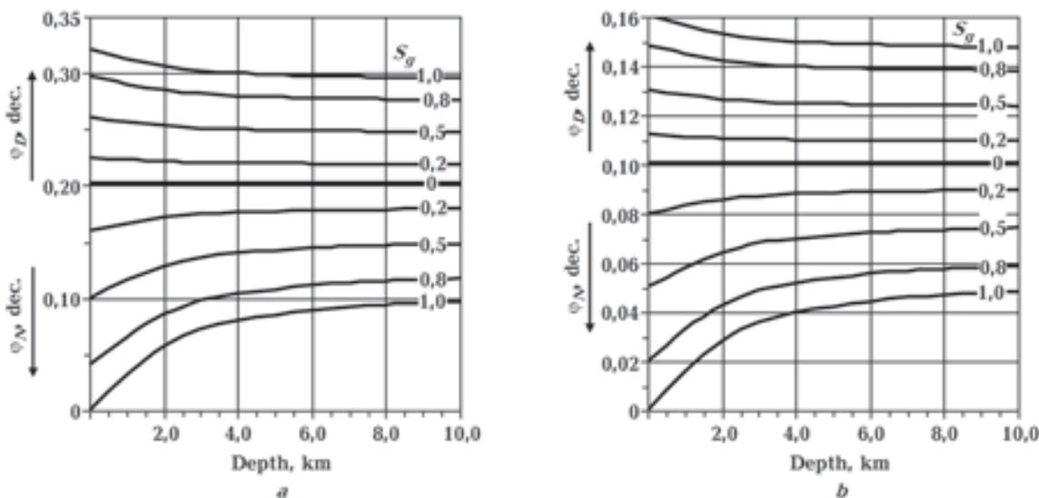
Fig. 1. Apparent porosities  $\phi_N$  and  $\phi_D$  of gas reservoirs vs depth for sandstone with  $\phi=0.2$  (a) and  $\phi=0.1$  (b) at different gas saturation.
