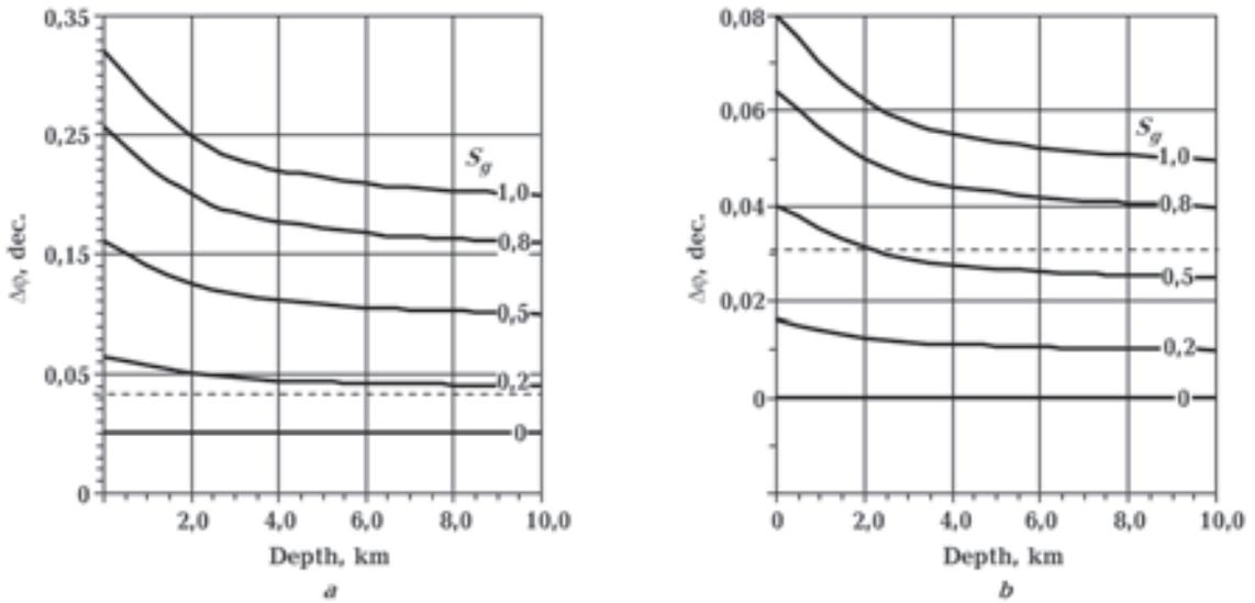
Fig. 3. Identification parameter  $\Delta\phi$  vs depth for sandstone with  $\phi=0.2$  (a) and  $\phi=0.05$  (b) at different gas saturation. Dashed line shows error of identification parameter.
