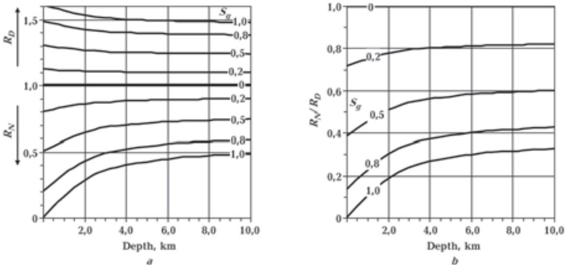
Fig. 2. Ratios  $R_D$ ,  $R_N$  (a) and  $R_N/R_D$  (b) vs depth for sandstone at different gas saturation.
