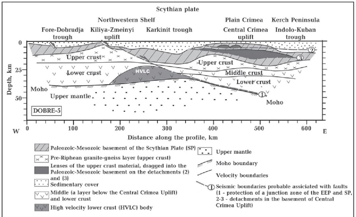
Fig. 1. Interpreted seismic model on the DOBRE-5 profile.
