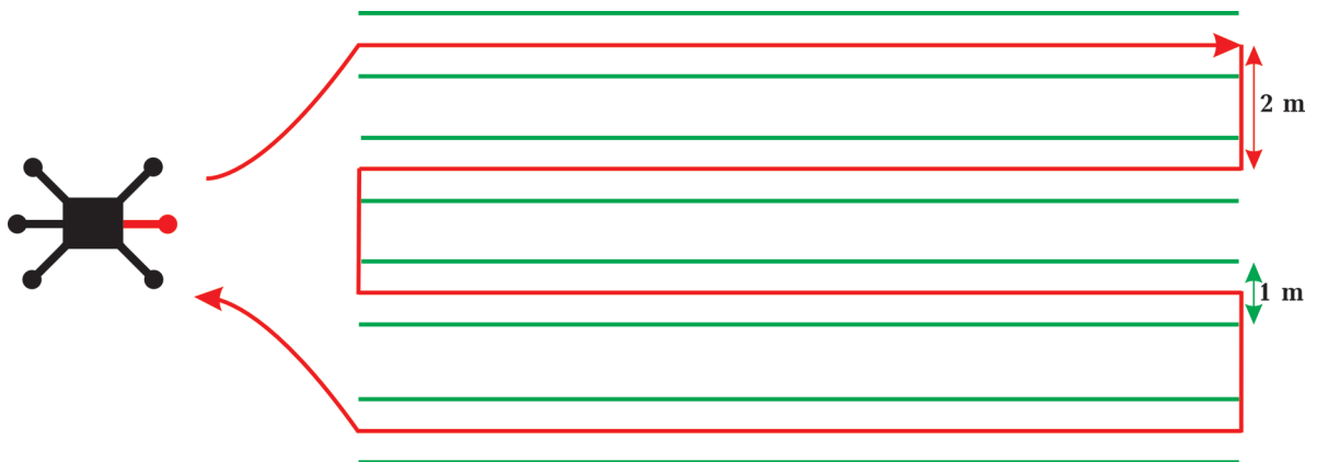
Fig. 5. An example of flight planning for magnetic surveying with a UAV. The red lines show the UAV flight profiles, and the green lines show the profiles along which the data are collected.
