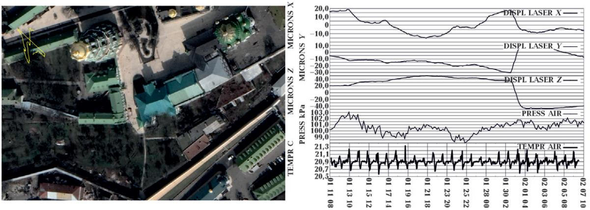
Fig. 13. Daily periodic displacements of the laser 3D inclinometer pendulum from 2024-01-21 00:06:44 to 2024-01-28 06:05:20 and plotted on the photo of building No. 3 on the map <http://lavra.igs-nas.org.ua/GoogleMaps/TST02/>.
