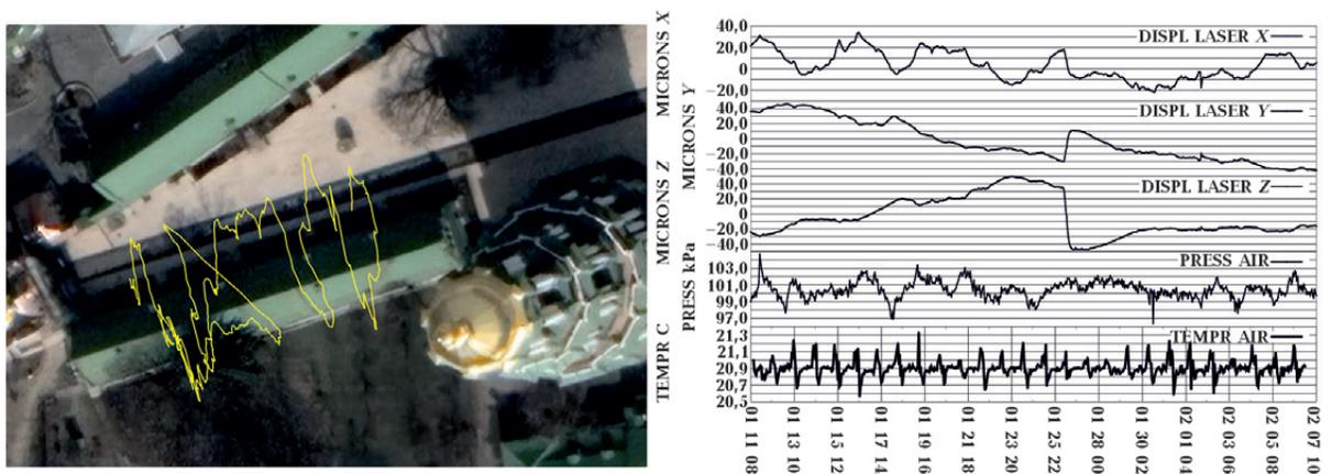
Fig. 12. Daily periodic displacements of the laser 3D inclinometer pendulum from 2024-01-11 13:06:31 to 2024-02-06 23:05:32 and plotted on the photo of building No. 3 on the map <http://lavra.igs-nas.org.ua/GoogleMaps/TST01/>.
