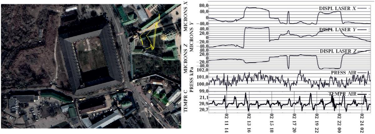
Fig. 14. Daily periodic displacements of the laser 3D inclinometer pendulum from 2024-02-10 00:05:02 to 2024-02-24 23:05:14 plotted on the photo of building No. 3 on the map <http://lavra.igs-nas.org.ua/GoogleMaps/TST03/>.
