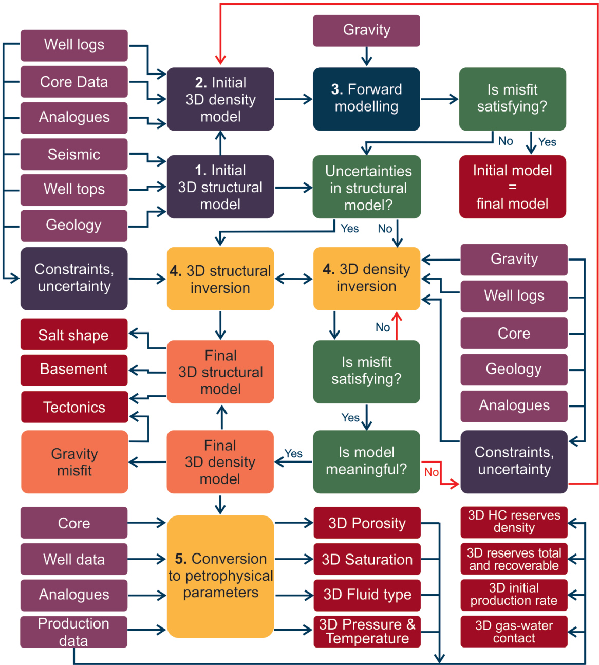
Fig. 1. Fundamental scheme of 3D joint inverse problem solution for gravity, well-log, seismic, and geological data, and estimation of petrophysical and hydrocarbon production properties of commercial hydrocarbon pools.
