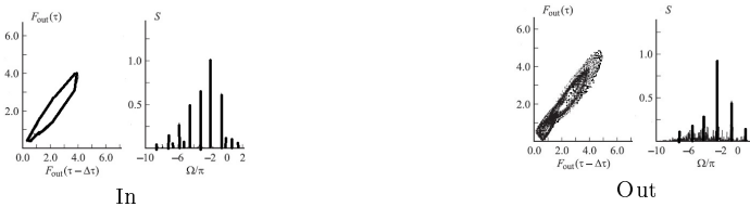
Fig.3. Temporal dependence of the output amplitude and signals spectrum: (In). input acting BWT; and (Out). Output BWT R=0.050 ;
