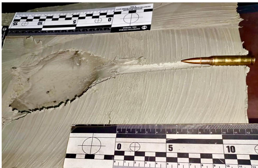
Fig. 8b. Residual cavity on firing a bullet with a steel core of caliber cartridge 7.62x51 mm NATO
