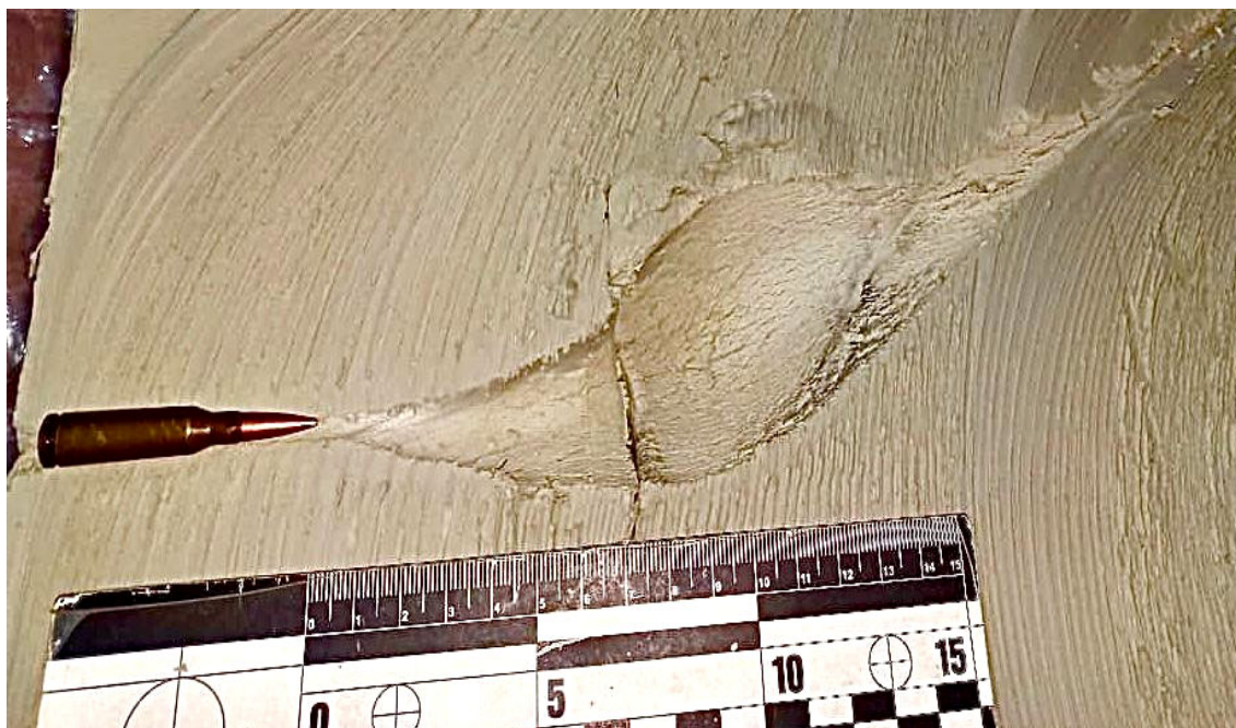
Fig. 7b. Residual cavity on firing a PS bullet of a military caliber cartridge 5.45x39 mm (7H6)
