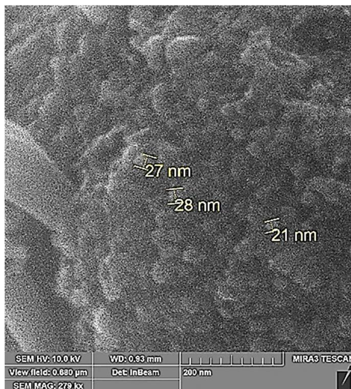
Fig. 1. Scanning electron microscope image of nano-TiO<sub>2</sub> at  $\times 279000$  magnification, a scale bar 200 nm
