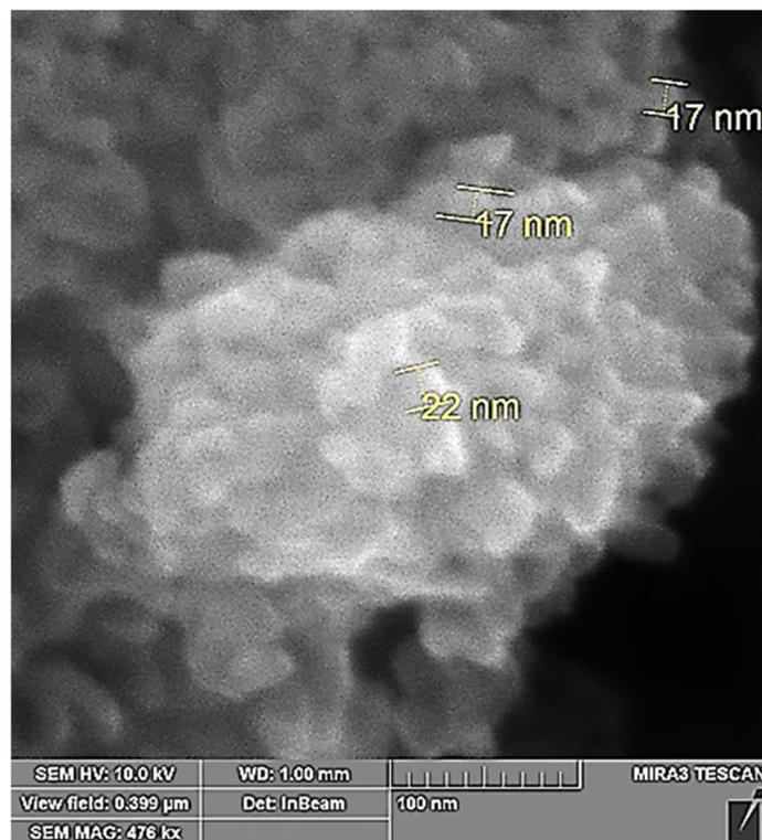
Fig. 2. Scanning electron microscope image of nano-TiO<sub>2</sub>@Ag at ×476000 magnification, scale bar 100 nm
