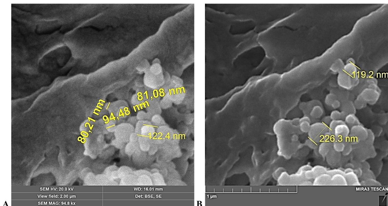
**Fig. 4. Results of SEM with nano-TiO<sub>2</sub> morphometry application.**
