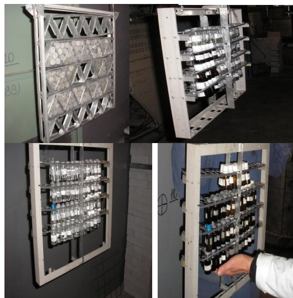
Fig. 2. Samples of monomers on the operation conveyer of radiation installation.
