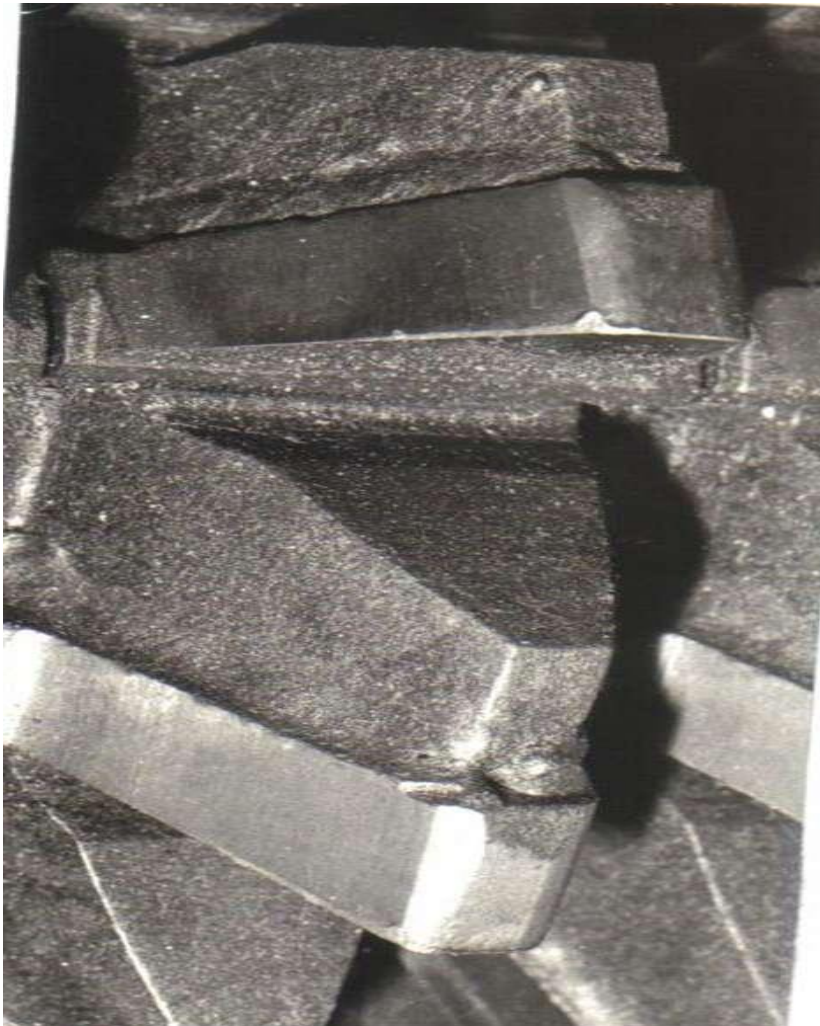
Fig. 10. Increased wear of the teeth of a finishing high-speed cutter of a pre-fabricated welded design
