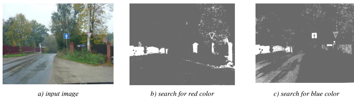
Fig. 6. Convert an image to search for colors that are specific to road signs
