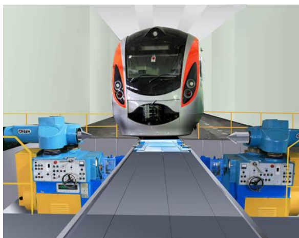
Fig. 1. Processing wheels without rolling out on a machine model KZh-20TF1
