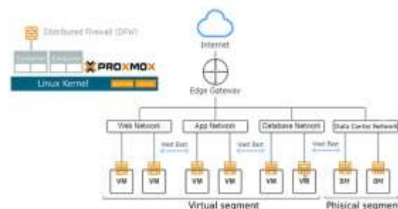
Fig. 1. Generalized diagram of a distributed firewall for a corporate network
