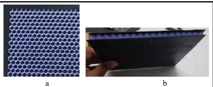
Fig. 2. Gluing of a three-layer panel: a – honeycomb structure with one sheathing; b – three-layer panel
