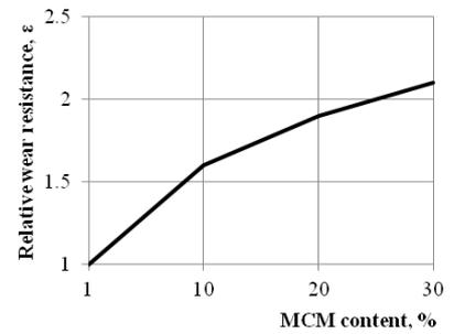
**Fig. 9. Relative wear resistance of layers deposited with composite material, depending on the MCM content**
