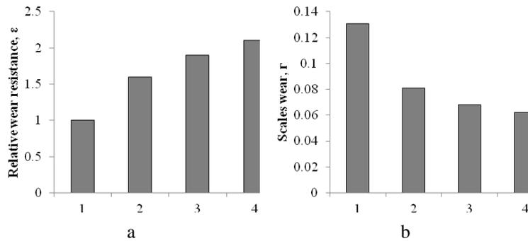
**Fig. 8. Wear resistance of deposited layers in the process of abrasive wear with unfixed abrasive:**
