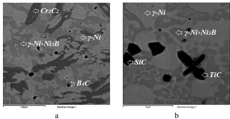
**Fig. 3. Microstructure and phase composition of deposited layers:**
