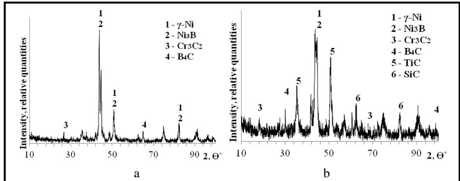
**Fig. 4. Diffractograms of deposited layers:**
