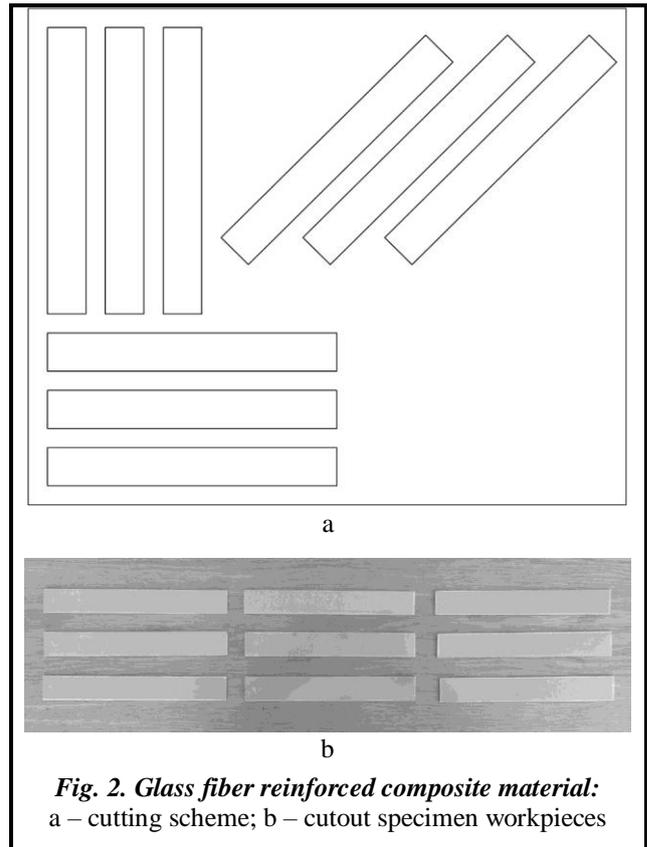
**Fig. 2. Glass fiber reinforced composite material:**
