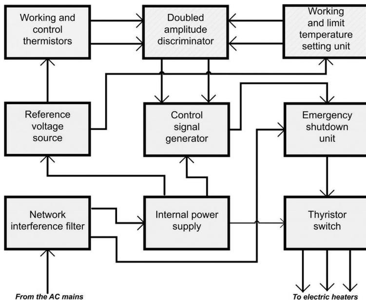
Fig. 6. Structural scheme of the ATCBEF
