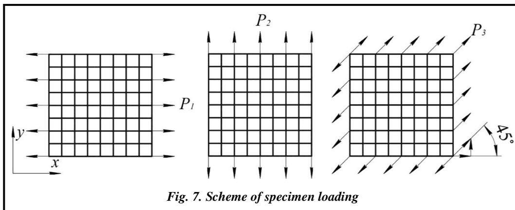
*Fig. 7. Scheme of specimen loading*
