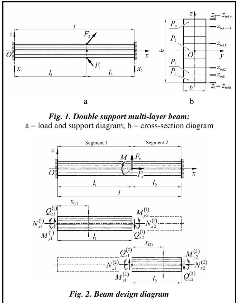
**Fig. 1. Double support multi-layer beam:**
