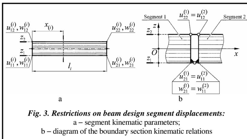
**Fig. 3. Restrictions on beam design segment displacements:**
