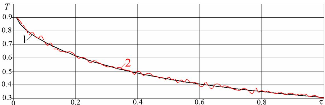
**Fig. 9. Temperature at the boundary of the plate with the required heat flux:**
