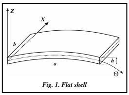
If we increase  $\eta_0$ , we can achieve such a value of this parameter that the radial displacements w  $(x, \theta, t)$  are comparable with the shell thickness h. Then a geometrically non-linear deformation will be observed. In this case, the deformations are small, and the movements are moderate. Since the deformations are small, then the components of stress and strain tensors satisfy Hooke's law.
