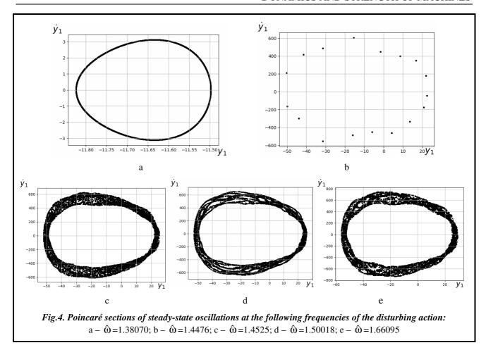
To study the steady-state oscillations, Poincaré sections, spectra of Lyapunov characteristic exponents, and spectral densities were analyzed, with the stroboscopic phase portrait used as Poincaré sections. The numerical methods for calculating the above three characteristics are covered in monograph [7].
