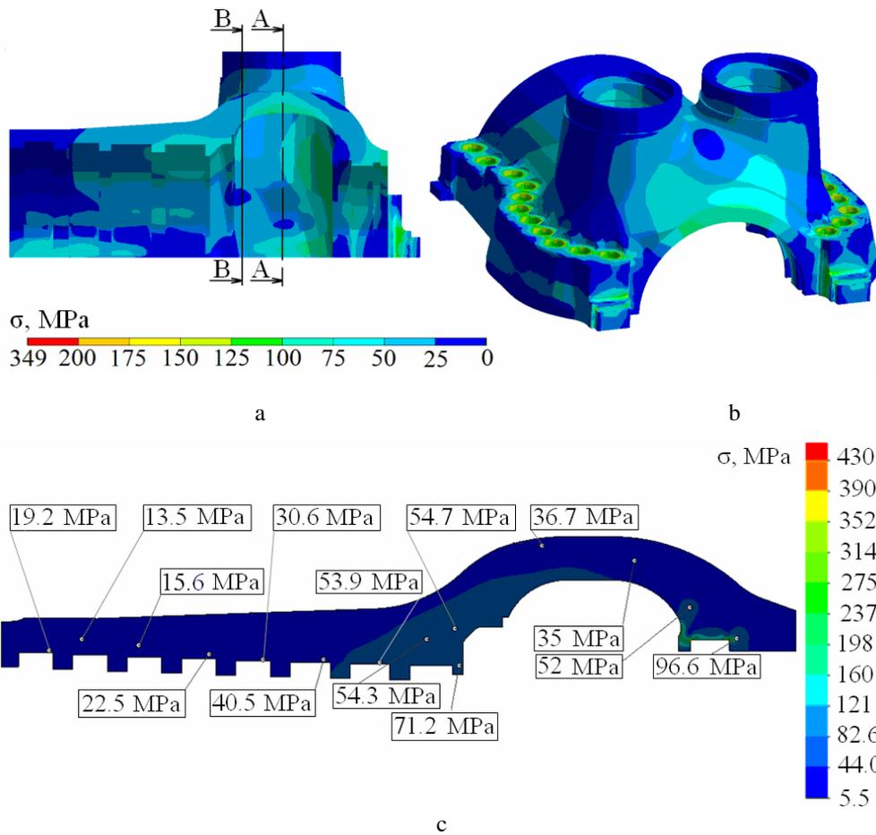
**Fig. 6. SSS of the internal HP casing for K-325-23.5 turbine:**
