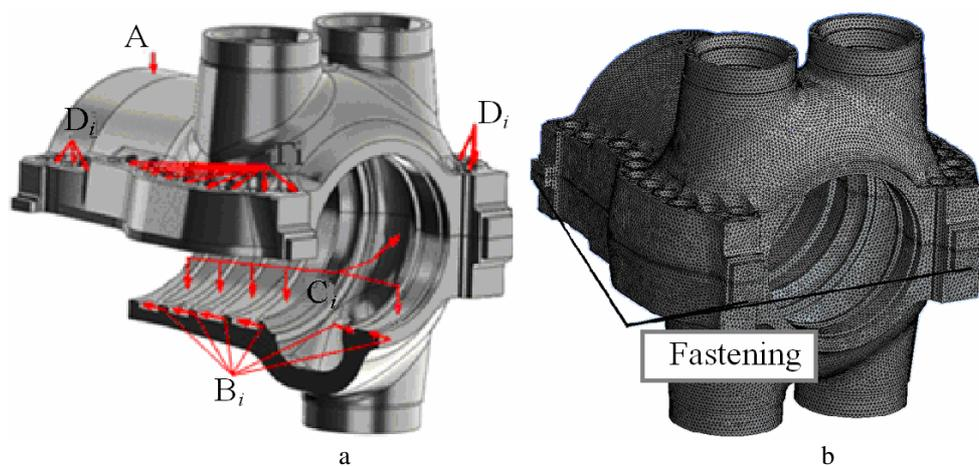
**Fig. 2. Computational model of the internal HP casing for the the K-540-23.5 turbine:**
