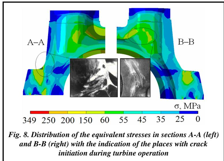
*Fig. 8. Distribution of the equivalent stresses in sections A-A (left) and B-B (right) with the indication of the places with crack initiation during turbine operation*
