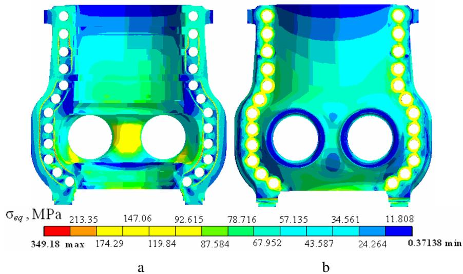
**Fig. 7. Distribution of the equivalent stresses on the internal HP casing:**
