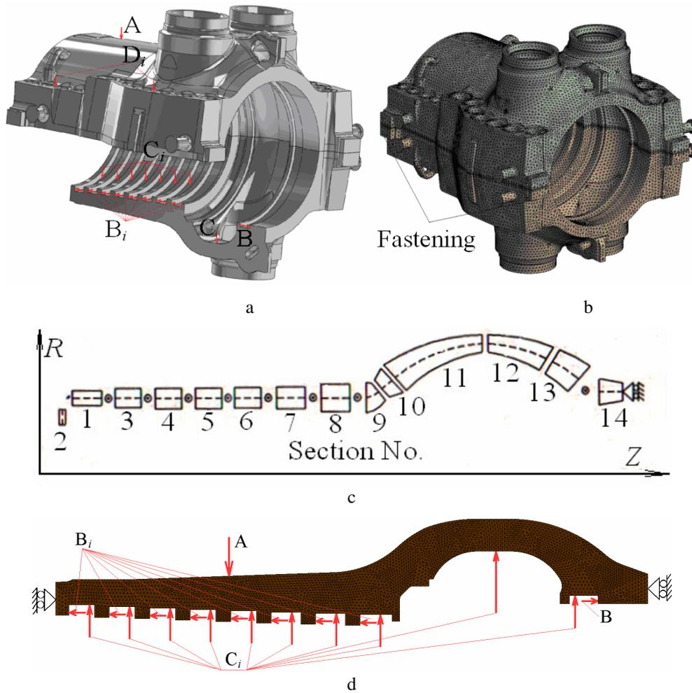
**Fig. 1. Computational models of the internal HP casing for the K-325-23.5 turbine:**
