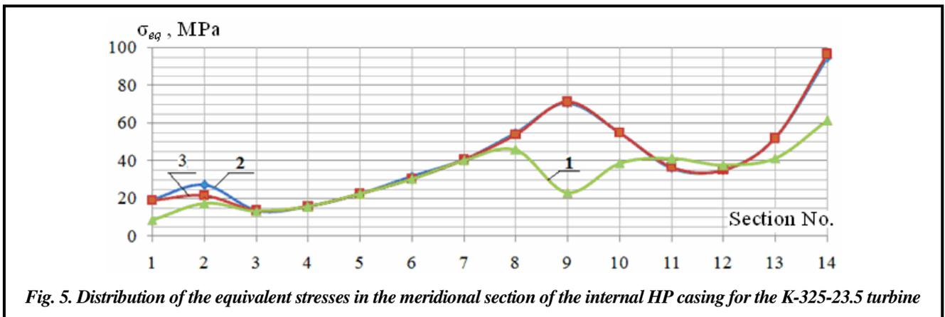
Fig. 5. Distribution of the equivalent stresses in the meridional section of the internal HP casing for the K-325-23.5 turbine
