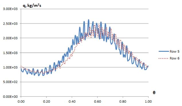
Fig. 18. Circumferential distribution of the specific flow rate for the rows # 5, 6 of the control section, 50% mode
