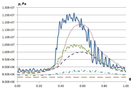
Fig. 15. Circumferential pressure distribution on the control section rows, 50% mode
