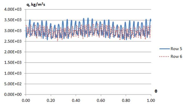
**Fig. 10. Circumferential distribution of the specific flow rate for the rows # 5, 6 of the control section, 100% mode**
