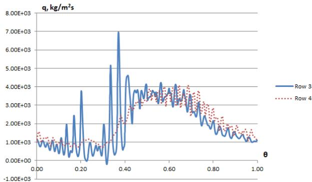
**Fig. 13. Circumferential distribution of the specific flow rate for the rows # 3, 4 of the control section, 70% mode**
