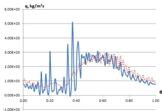
Fig. 17. Circumferential distribution of the specific flow rate for the rows # 3, 4 of the control section, 50% mode
