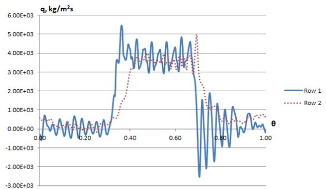
Fig. 16. Circumferential distribution of the specific flow rate for the rows # 1, 2 of the control section, 50% mode
