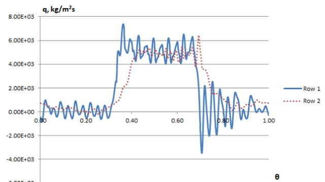
**Fig. 12. Circumferential distribution of the specific flow rate for the rows # 1, 2 of the control section, 70% mode**
