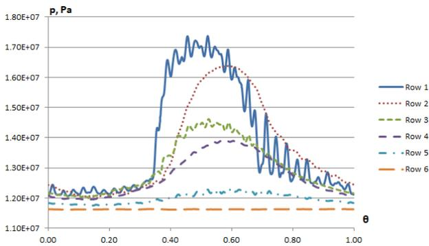
**Fig. 11. Circumferential pressure distribution on the control section rows, 70% mode**
