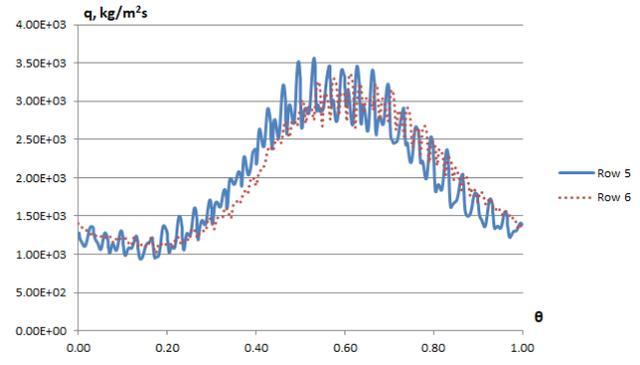
**Fig. 14. Circumferential distribution of the specific flow rate for the rows # 5, 6 of the control section, 70% mode**
