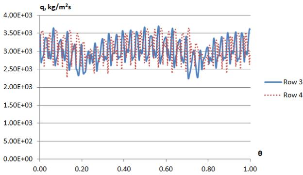
**Fig. 9. Circumferential distribution of the specific flow rate for the rows # 3, 4 of the control section, 100% mode**
