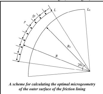
At the straight ends of the friction lining, the boundary conditions are accepted as
