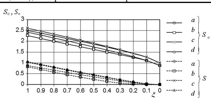
Fig. 3. Optimization results for I-beam element flanges
