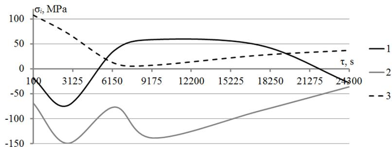
**Fig. 4. Dynamics of changes in stress intensity in the IPC CV at start-up from the cold thermal state**
