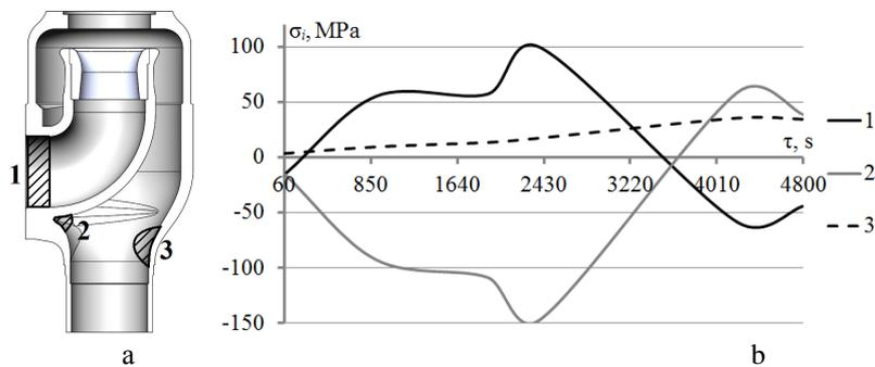
**Fig. 3. Dynamics of changes in stress intensity in the IPC CV at start-up from the hot thermal state:**
