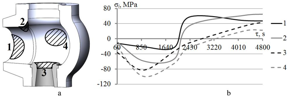
**Fig. 1. Dynamics of changes in stress intensity in the HPC CV at start-up from the hot thermal state:**
