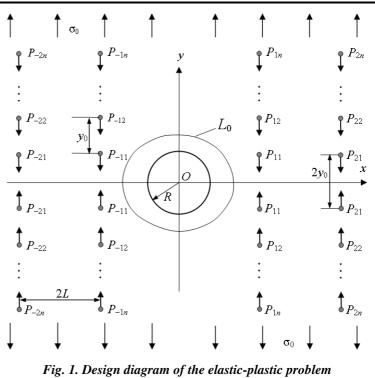
Fig. 1. Design diagram of the elastic-plastic problem for a stringer plate
