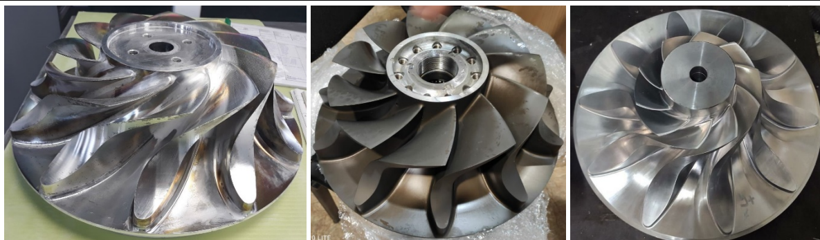
Fig. 16. Examples of developed and implemented TEU turbine rotors
