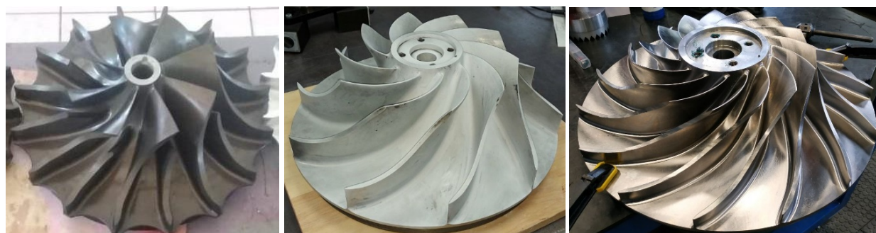
Fig. 17. Examples of developed and implemented TEU compressor rotors
