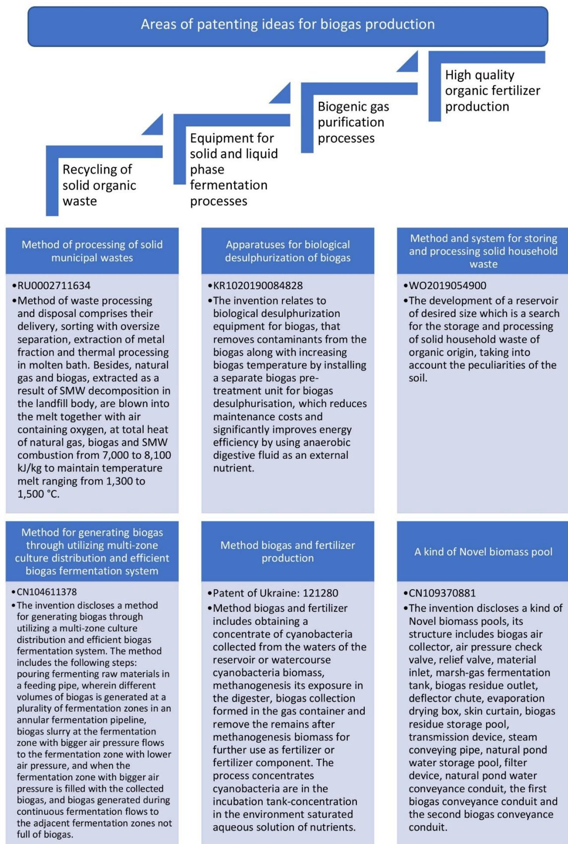
Fig. 5 – An overview diagram of the analysis of patent databases on the topic “Methods of producing biogas”
