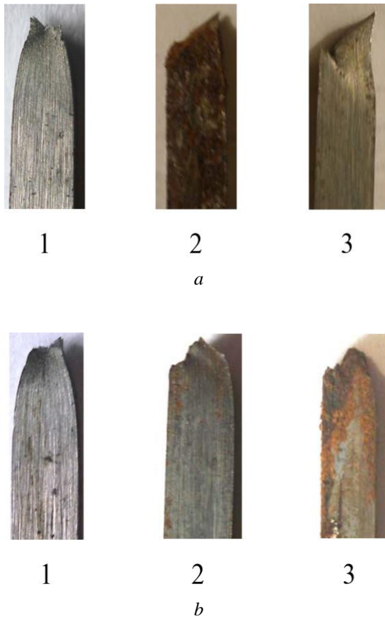
Fig. 7. Photos of fractures of the X70 pipe steel samples made from the pipe A and the pipe B after mechanical tests in air and corrosion-mechanical tests in the solution at the influence of a complex of stress-corrosive factors at the potential -2.0 \text{ V}_{\text{Ag}/\text{AgCl}} :
