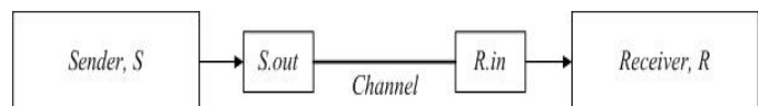
Fig.7. Example of interaction between two network elements (sender and receiver), unidirectional communication channel
