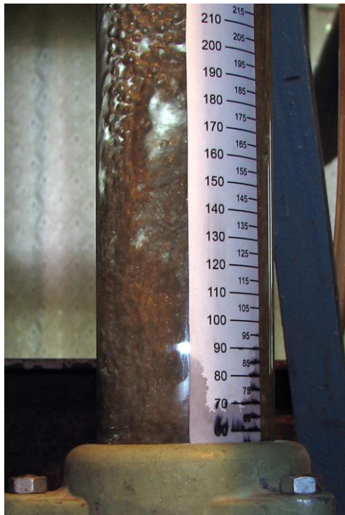
Fig. 3. Regime of mobile gas-liquid layer: tray # 21 (table 1) L=13,5 \text{ m}^3/(\text{m}^2 \cdot \text{h}) , w=1,44 \text{ m/s}
