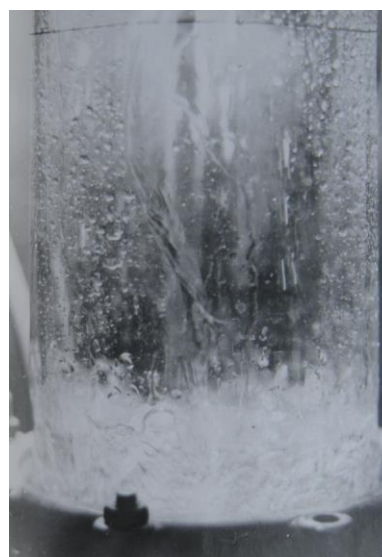
Fig. 2. Regime of continuous barbotage layer: tray # 10 (table 1) L=12,7 m 3 /(m 2 ·h), w=0,72 m/s
