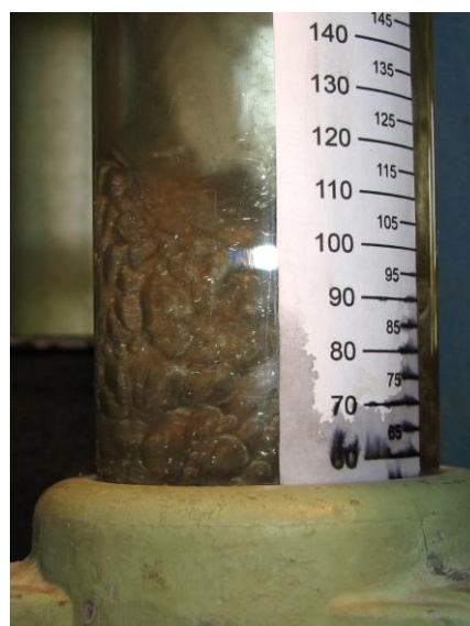
Fig. 1. Regime of continuous barbotage layer: tray # 21 (table 1) L=13,5 m 3 /(m 2 ·h), w=0,56 m/s
