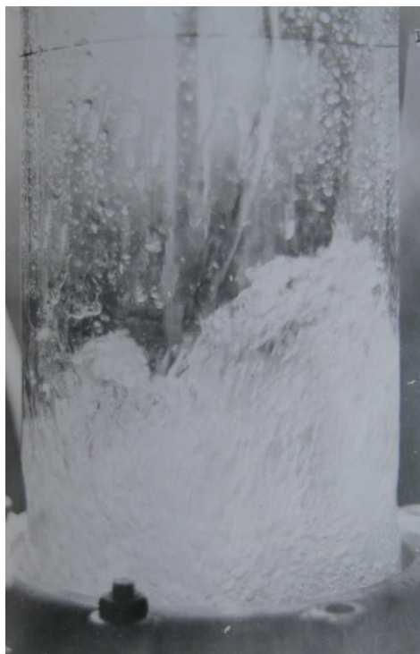
Fig. 4. Regime of mobile gas-liquid layer: tray # 10 (table 1) L=12,7 \text{ m}^3/(\text{m}^2 \cdot \text{h}) , w=0,83 \text{ m/s}
