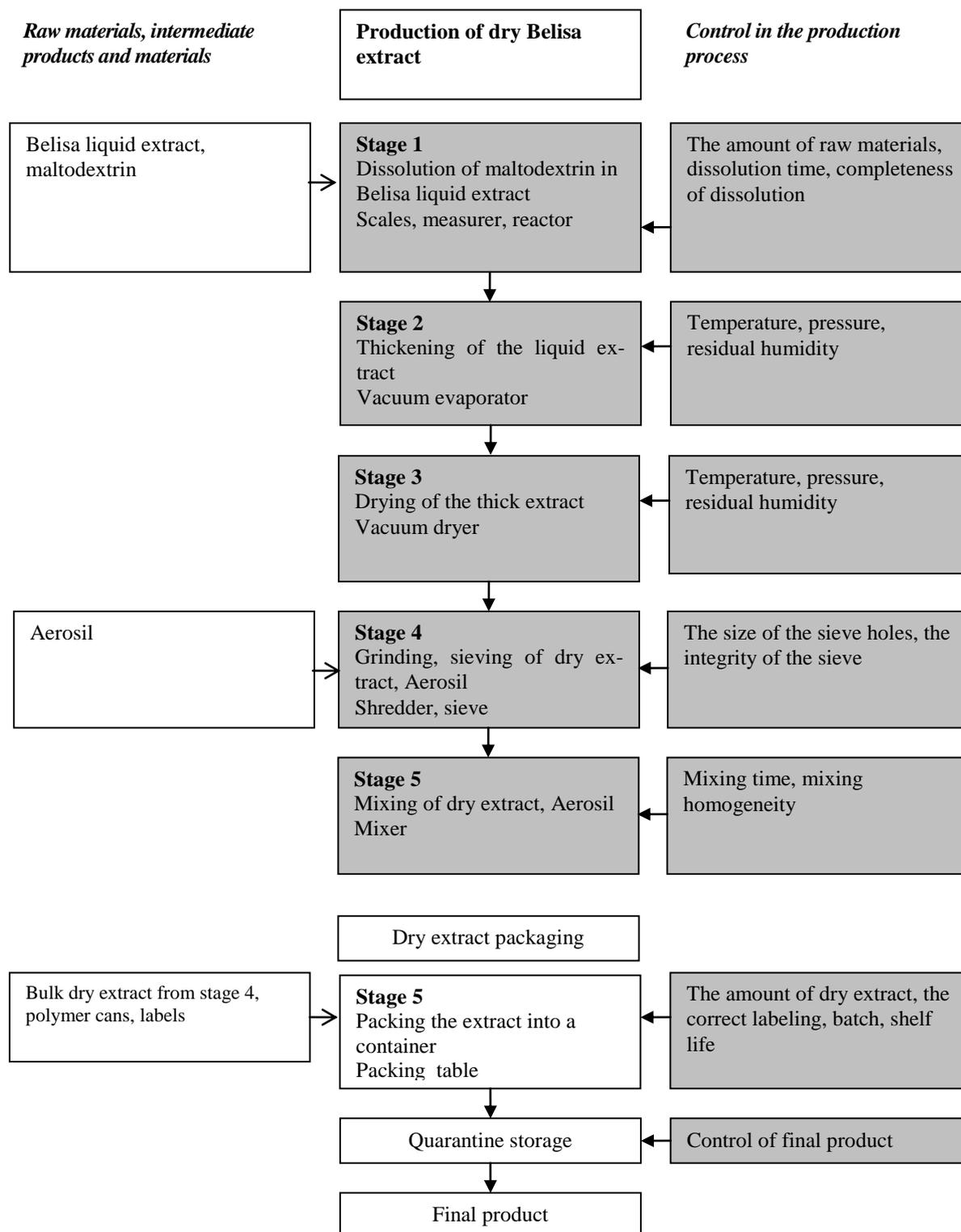
Fig. 3. Technological scheme of production of dry Belisa extract (sample No. 7)
