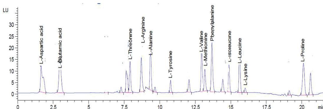
Fig. 8. The chromatogram of free amino acids of dry extract of *C. mollis* leaves
