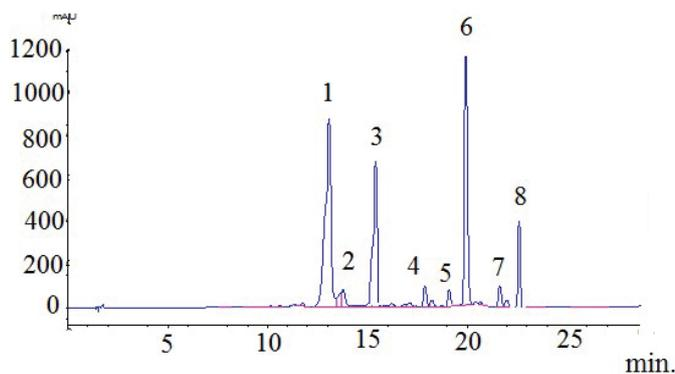
Fig. 5. HPLC chromatogram of phenolic compounds of dry extract of *C. mollis* leaves
