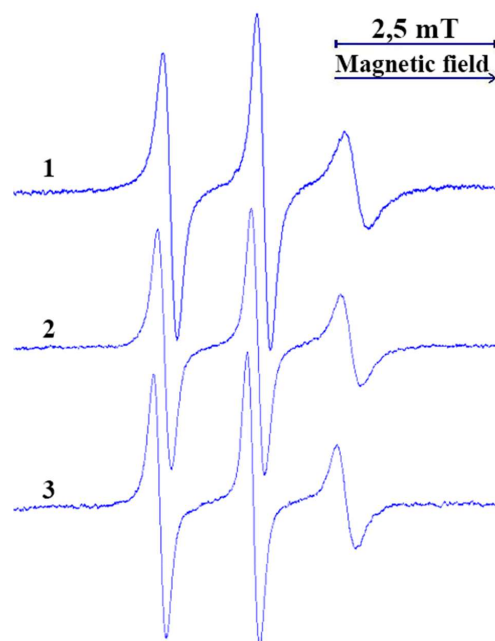
Fig. 6. Representative EPR spectra of hydrophilic probe 2 in 20 % P338 solution at 1 – 25 °C, 2 – 32 °C, 3 – 37 °C
