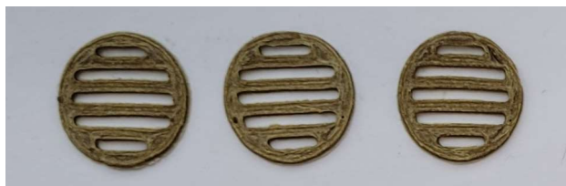
Fig. 6. The semi-solid extrusion (SSE) 3D-printed round-shaped discs ( n=3 ). The printed discs were prepared from the functionalized polyethylene oxide (PEO) gel (Sample 1) loaded with 1,2,3-triazolo-1,4-benzodiazepine nanofibers and a valine-modified motherwort herb dry extract. Reference is also made to Table 1
