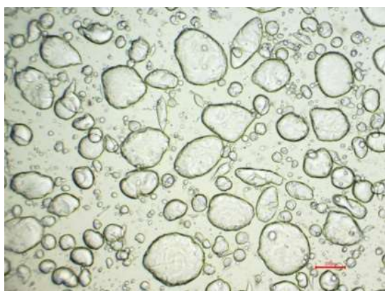
Fig. 2. Photomicrograph of the first stage of soap formation
