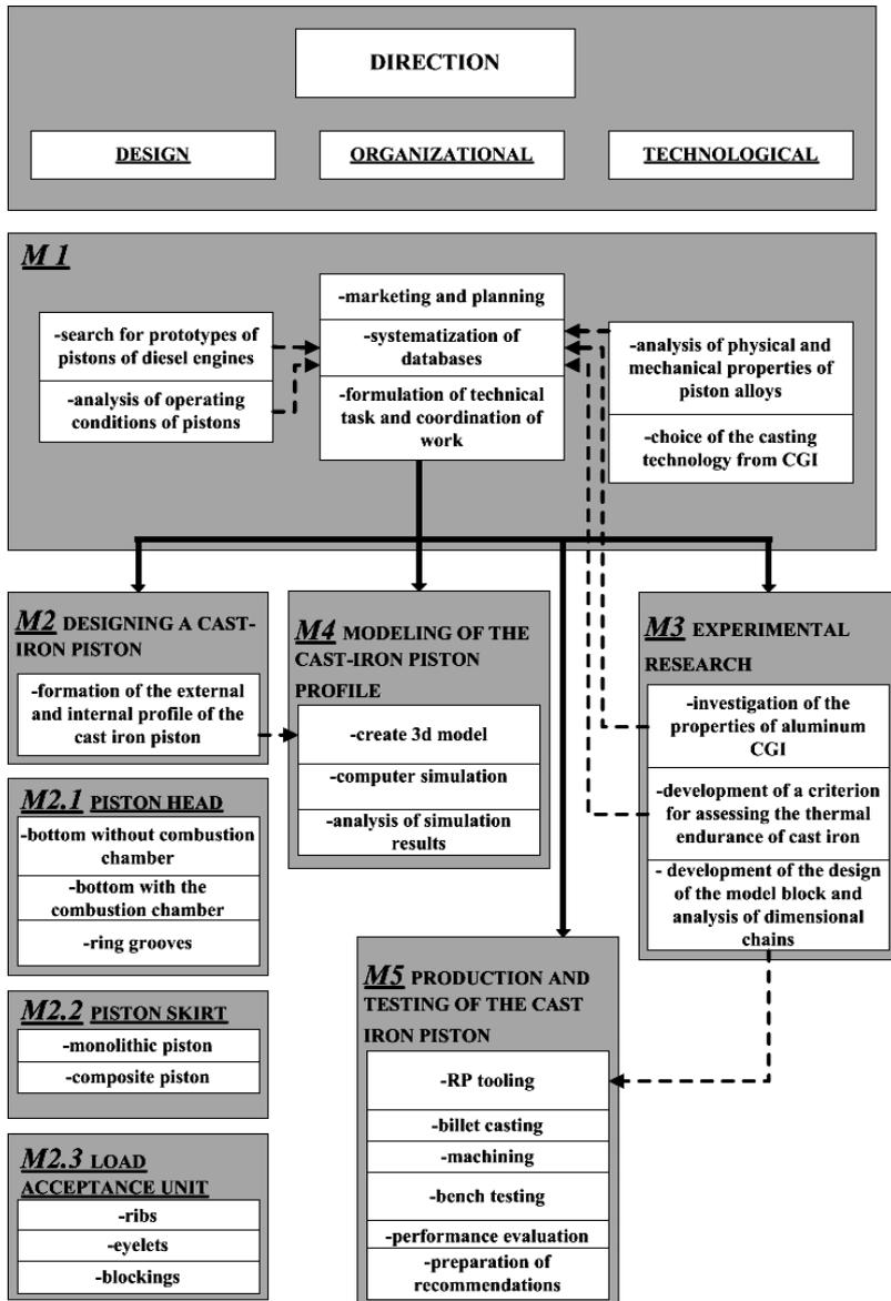
Fig. 1. System for organizing the modular design of cast-iron pistons for internal combustion engines
