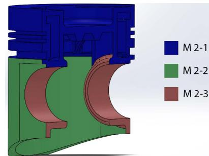
Fig. 2. Projected zones of the piston
