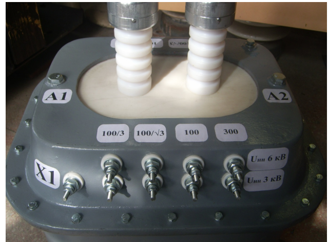
Fig. 1. 10 kV class high-voltage autotransformer. View from the side of 3 kV and 6 kV windings
