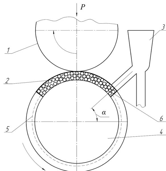
Fig. 1. Welding scheme for metal powder: 1 – roller-electrode; 2 – welded layer; 3 – bunker; 4 – part; 5 – mesh; 6 – powder
