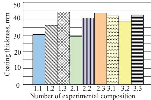
**Fig. 5.** The thickness of the fire-resistant coating of different compositions after the experiments
