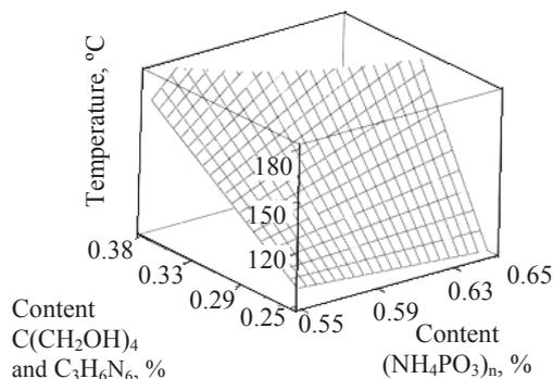
**Fig. 7.** The dependence of temperature on a back surface of the sample from content of composition
