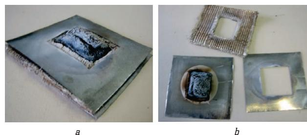
**Fig. 2.** Experimental sample after fire resistance testing:
