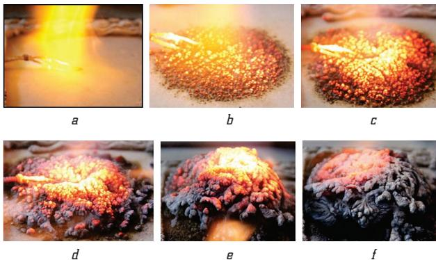
**Fig. 4.** Change of samples surface with a fire resistant coating when exposed to a flame during a time  $\tau$  at a temperature on a back surface  $T$ :
