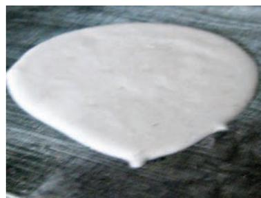
**Fig. 1.** Sample of fire-resistive coating
