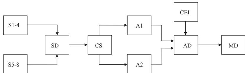
**Fig. 2.** Structural diagram of a three-channel measuring system measurements of dipole magnetic moments: S1-4 – sensors of the first group; S5-8 – sensors of the second group; SD – switching device; CS – channel switch; A1, A2 – amplifiers; AD – adder; CEI – compensator of external interference; MI – measuring device
