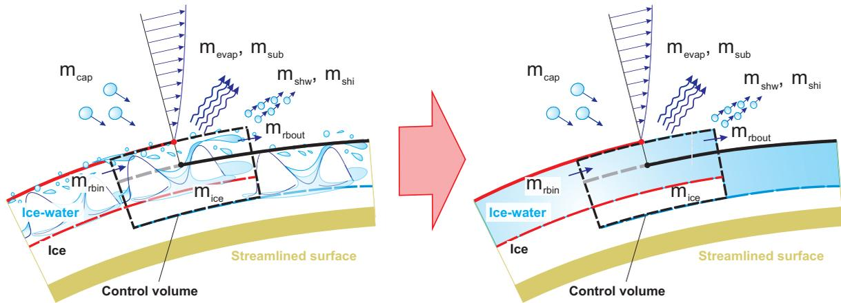
Fig. 4. Scheme of transition to a mathematical model of ice growth
