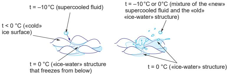
**Fig. 1.** The temperature distribution on the streamlined surface (in the conditions of the experiment conducted:  $t_{\infty} = -10\text{ °C}$ ,  $v_{\infty} = 33\text{ m/s}$ ,  $LWC = 2.4\text{ g/m}^3$ ,  $d_k = 150\text{ microns}$ )
