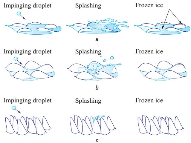
**Fig. 3.** The effect of temperature on the mechanism of movement and subsequent solidification of surface moisture: a - 2.5 °C; b - 10.0 °C; c - 15.0 °C (under the conditions of the experiment conducted:  $v_{\infty} = 33\text{ m/s}$ ,  $LWC = 2.4\text{ g/m}^3$ ,  $d_k = 150\text{ microns}$ )
