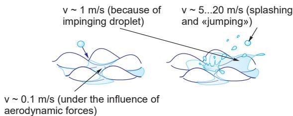
**Fig. 2.** The mechanism of fluid movement along a streamlined surface (under the conditions of the experiment conducted:  $t_{\infty} = -10\text{ °C}$ ,  $v_{\infty} = 33\text{ m/s}$ ,  $LWC = 2.4\text{ g/m}^3$ ,  $d_k = 150\text{ microns}$ )
