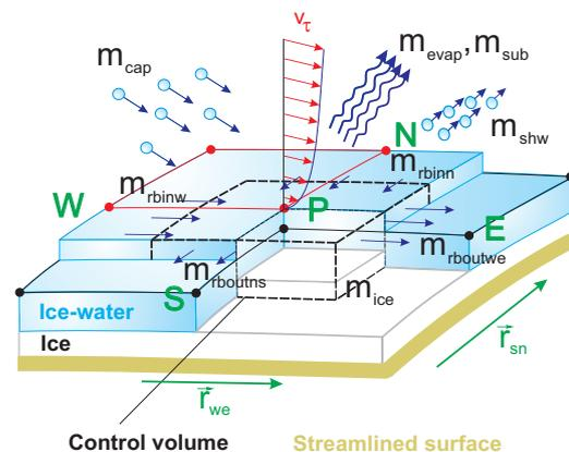
Fig. 5. Scheme of mass flows in the control volume
