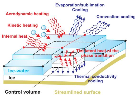
Fig. 6. The scheme of heat flows in the control volume
