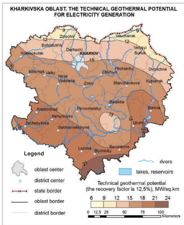
Fig. 4. Technical potential of the geothermal resources of the Kharkiv region (oblast) for the electricity generation
