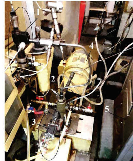
Fig. 6. Fuel injection system with sensors on non-motorized stand: 1 – nozzle; 2 – HPFP; 3 – device that controls the displacement of the fuel pump rack; 4 – electric motor; 5 – motor control station
