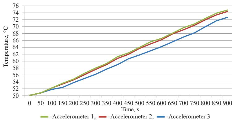
**Fig. 4.** Changes in the average temperature over the accelerometer volume in time (option 2)
