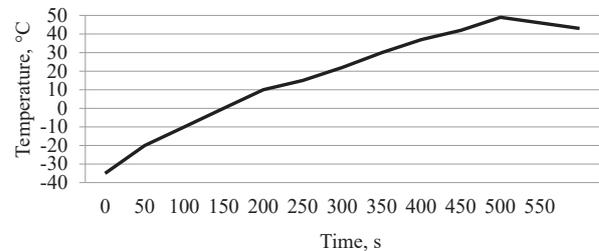
**Fig. 3.** Changes in the average temperature over the volume of the gyro sensor in time (option 1)
