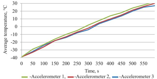
**Fig. 2.** Changes in the average temperature over the accelerometer volume in time (option 1)
