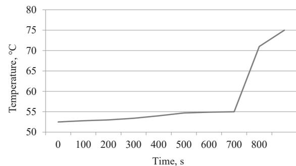
**Fig. 1.** The change in ambient gas temperature during the preparation of a remote measurement device in the coordinate measuring machine
