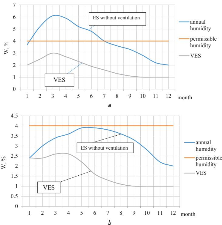
**Fig. 3.** Distribution of moisture inside the open enclosing structure (VES):
