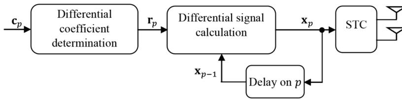
Fig. 2. The structural diagram of the encoder of differential space-time block coding (DSTBC)
