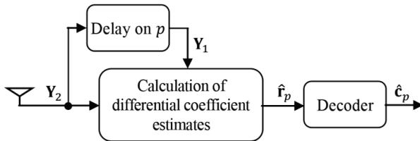
**Fig. 4.** The structural diagram of the differential spatial-temporal block coding (DSTBC) decoder
