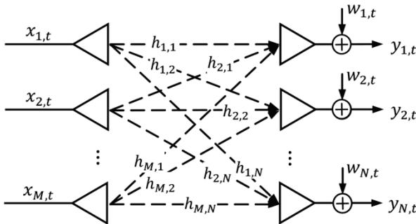
**Fig. 1.** Block diagram of a multi-antenna radio communication system (MIMO)
