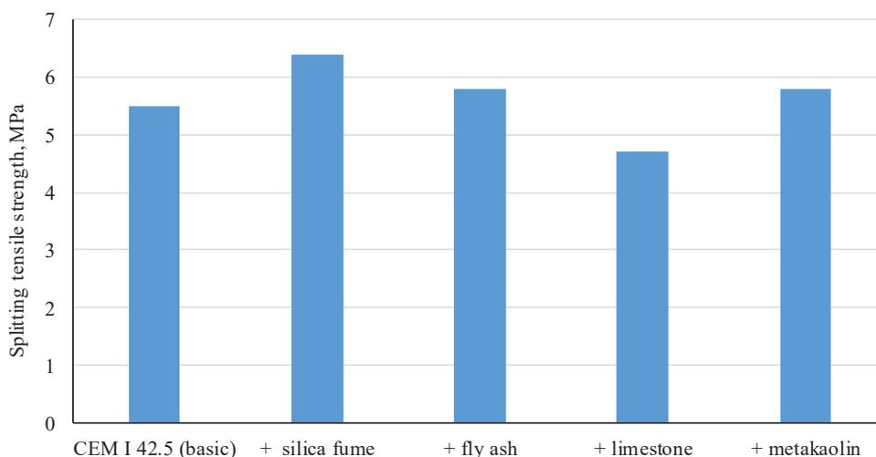
**Fig. 4.** Splitting tensile strength of high-strength concrete
