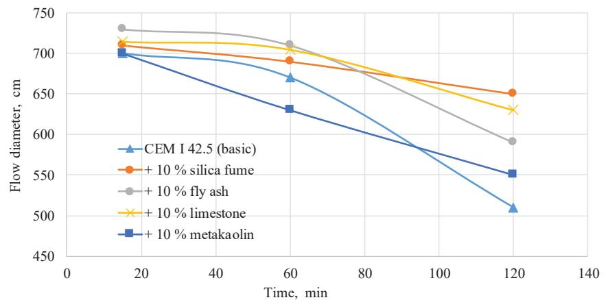
Fig. 1. Flow diameter of concrete mix in time
