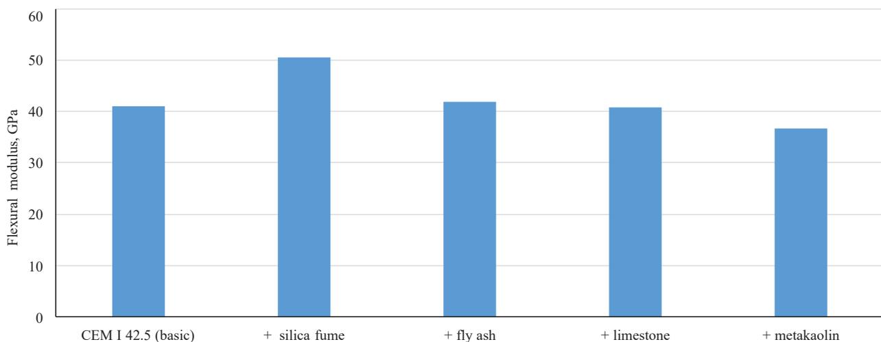
Fig. 7. Flexural modulus of the investigated concretes
